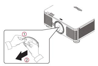
2. Align the "♠ " symbol on the lens label with the "\* " symbol on the top of the body (align to the center of the lens hole) and pull in the lens.
