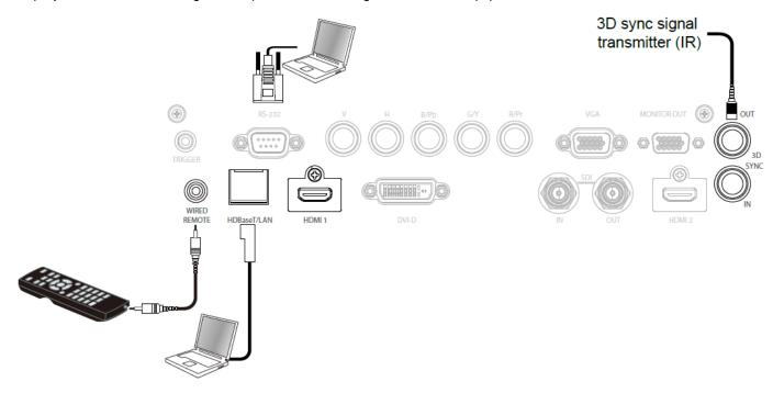
**HDBaseT/LAN (Network control):** The projector supports network control. LAN and HDBaseT share the one port. If only network control is used, you can connect the LAN on the projector to PC or through the local network. Refer to the Remote Communication Manual for detailed information.
