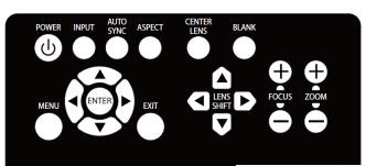
To open the OSD, press the Menu button on the OSD control panel or remote control. There are five folders on the menu. Press the cursor ◀ or ▶ buttons to move through secondary menus.
